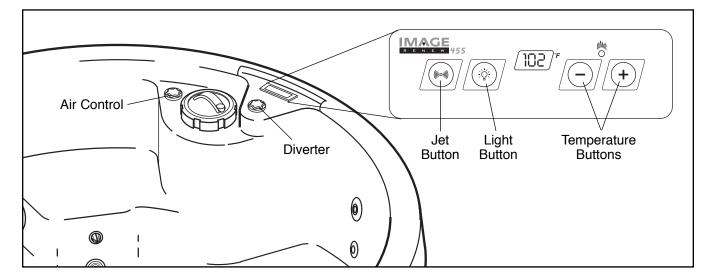
Refer to the diagram above. The function of each control is explained below:
